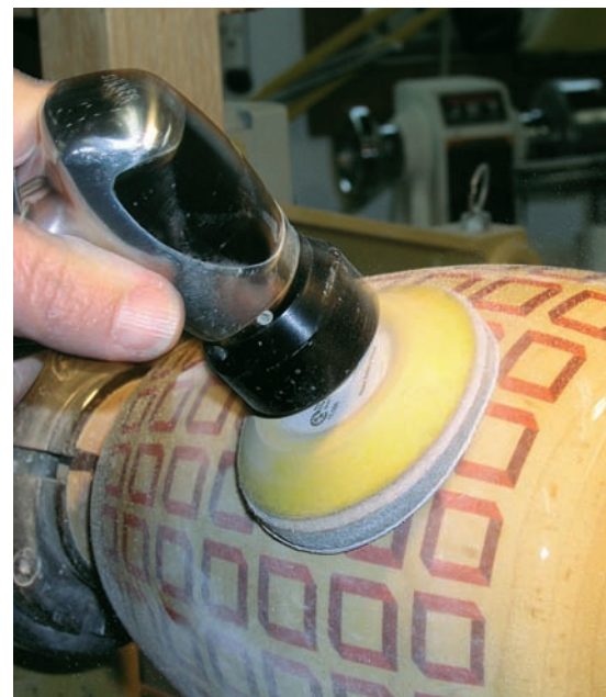
A 3" 3M 260L disc levels and prepares a varnished work for the next coat of Steve Sinner's vessel. The air-powered random-orbit sander is coupled with a ½" soft interface pad for sanding curves.
