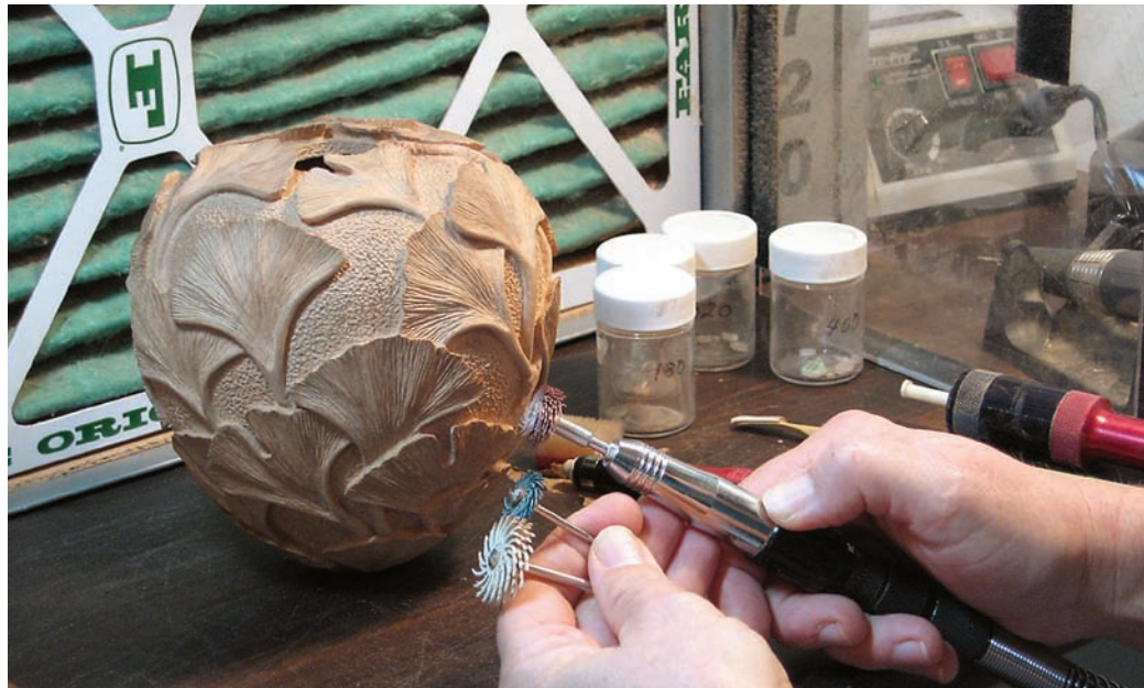
Dixie Biggs shows an assortment of 3M Bristle Discs and the flexible shaft tool she uses to drive them. Also shown is the Pfingst Micro Sander, with spare discs in the jars. Note Dixie's dust-collection hood—an essential protection for her respiratory system.
