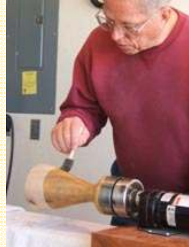
Applying the Polyurethane as the machine revolves.
