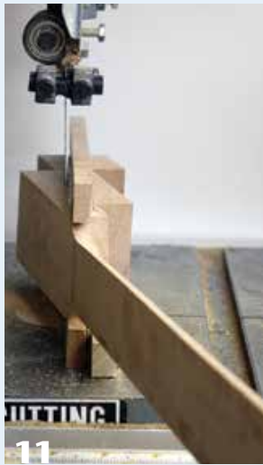
11 The side strips, glued at 13° from the neck line, act as a cutting guide.
