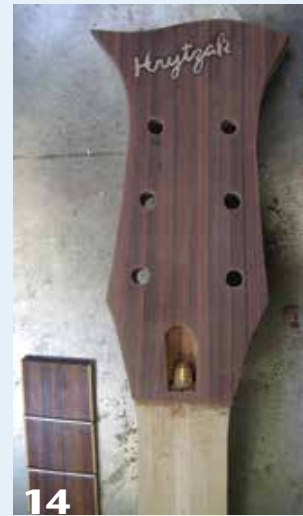
13 A template for locating holes for the tuning machines helps in determining the final shape of the peghead, whose rosewood veneer matches the fingerboard.
