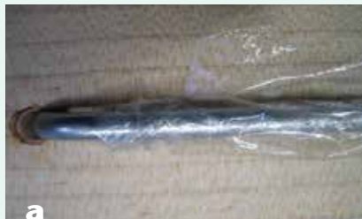
a A neck-embedded truss rod, here ready to be set in its groove, allows for straightening of a bent neck. The rod lies in a dado in the neck under the fingerboard. Plastic wrap prevents the rod from becoming glued in place.
