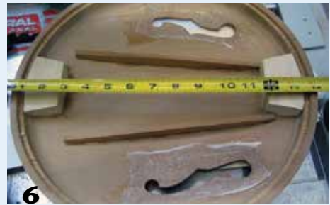
6 Inside the soundboard, with f-shaped sound holes, reinforcing blocks, and tuning bars that also act as bracing.
