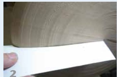
2 I used profile gauges made of cardboard to get the soundboard and backboard profiles correct during turning.
