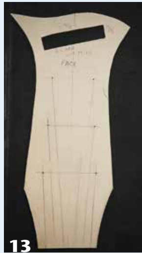
13 A template for locating holes for the tuning machines helps in determining the final shape of the peghead, whose rosewood veneer matches the fingerboard.
