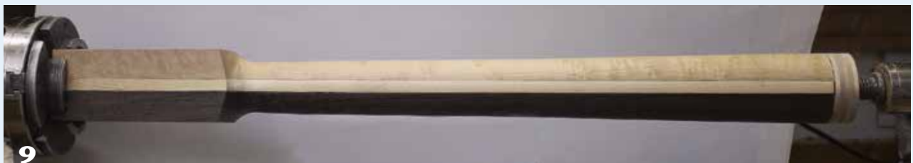
The neck blank is a split turning that comprises stock for two necks plus a spacer between them, resulting in necks shallower than a half circle. A plywood waste block at the tailstock end prevents the live center from splitting the assemblage, glued only near the ends.
