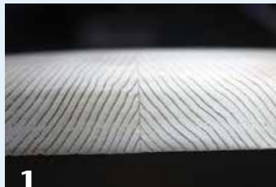
1 The alignment of the growth rings is critical for the strength of the soundboard.
