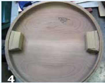
4 Reinforcing blocks are glued in position in the backboard to provide strength to the neck and tailpiece areas.
