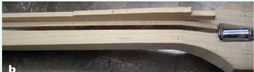
b A wood filler strip, here ready to be glued in, covers the truss rod and provides backing support during tensioning. A threaded portion of rod protrudes into the peghead for adjustment. A socket wrench confirms access to the rod's tensioning nut.
