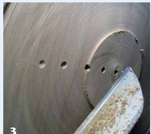
3 Predrilled depth holes aid in achieving thickness variations.
