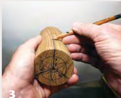
Extend the section lines down the cylinder to the opposite end, either freehand or with the aid of the toolrest. Locate and punch the three turning points at the opposite end, and label them as you did the first end.
