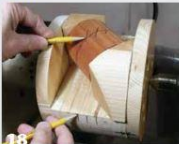
18 Mark a centerline, then use the true width of cut to mark the edges of the first cove.
