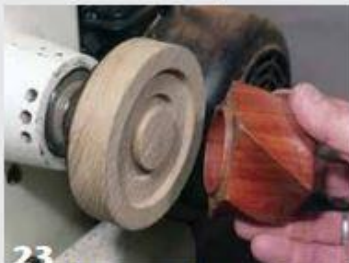
23 To finish the top to a nicely rounded dome, mount it on a tightly fitting plug chuck and anchor with hot-melt glue.
