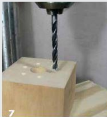
7 Use the index template to mark locations and bore a ring of six ¼" holes around the centered ¼" hole.
