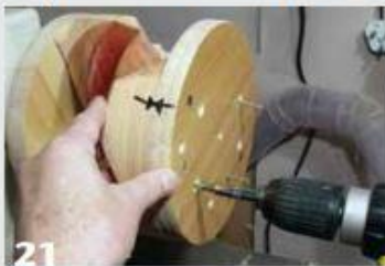
21 Undo the tailstock disk to rotate the blank one index position for the next coved face.
