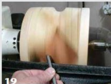
19 Turn the first cove to the marked edges. The cove will be cut into the jig along with the workpiece.
