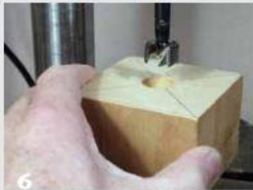
6 Bore a centered ¼" hole completely through the index block.
