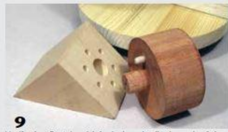
9 Verify that Part A, with its index pin, fits in each of the block's six positions.
