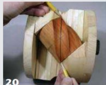
20 The deepest cut along the centerline completes the top and bottom edges of the twisted face. Sand the cove by hand before turning the next face, or cove.
