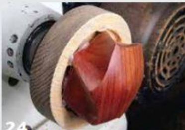
23 To finish the top to a nicely rounded dome, mount it on a tightly fitting plug chuck and anchor with hot-melt glue.
