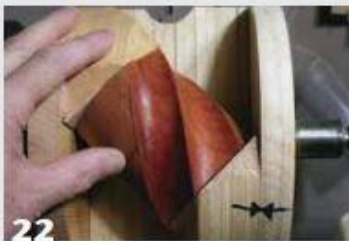
22 The profile just cut into the offside block now guides the second and subsequent cuts.
