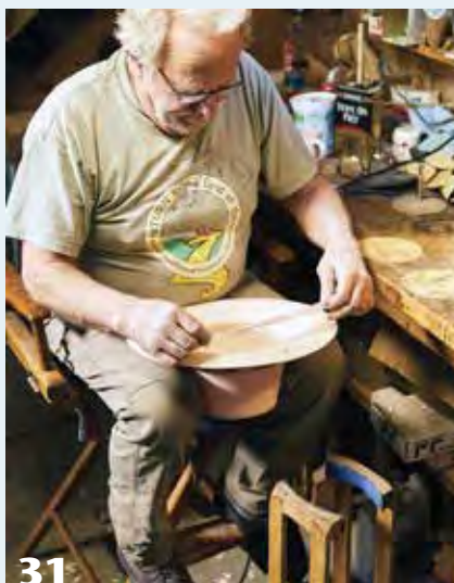
Apply tape over the two endgrain portions of the hat to help prevent cracking in these areas.
