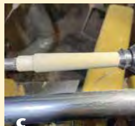
(b) Outboard side: Locking pliers grip the lamp rod next to the wood centering plug, preventing the rod from rotating with the spindle.
