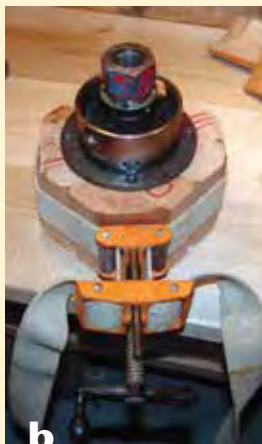
(b) The bevels align the wood jaws into an octagon. Pre-drill and use long screws to attach the wood to the jaws.
