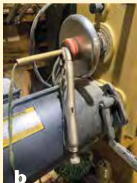
(b) Outboard side: Locking pliers grip the lamp rod next to the wood centering plug, preventing the rod from rotating with the spindle.
