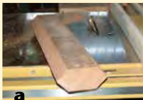
(a) A 24"-long board with ripped 45-degree bevels.
