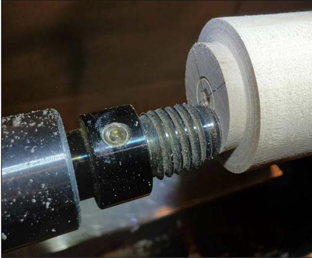
**Photo 2.** After turning the blank to a rough cylinder, establish the secondary axis by moving the center at the headstock end. The offset distance need not be exact, but the author uses the diameter of her cup drive as a handy measurement.
