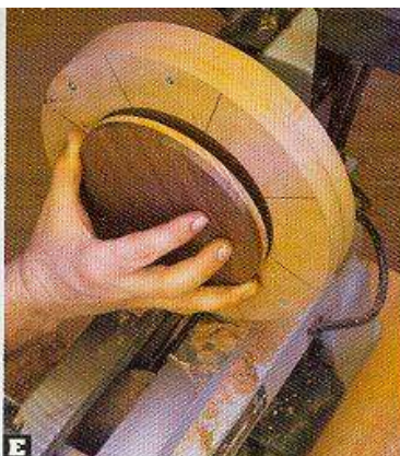
Tool: Parting tool Tool Rest: Center Speed: 800–1,200 rpm
