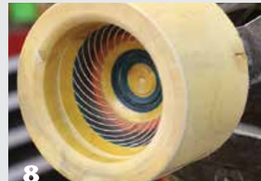
8 The box lid, ready for female threads.
