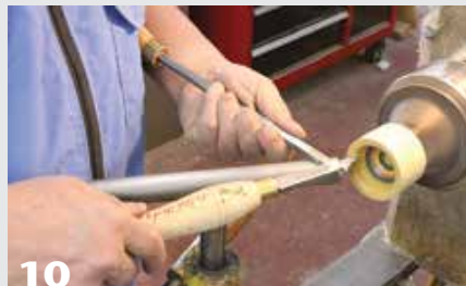
9 The female thread chaser is used with the armrest tool to form interior threads. An initial groove in the chamfer acts as a starting point for cutting the threads. Note that the chaser tool progresses to parallel with the bed ways as the threads develop.
