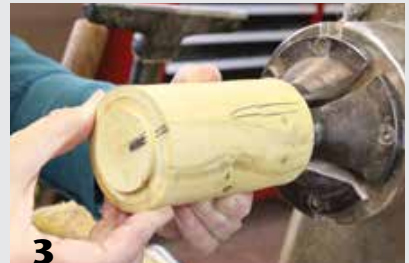
3 Hold the base up to the lid with the grain aligned and make registration lines to help with realignment later.
