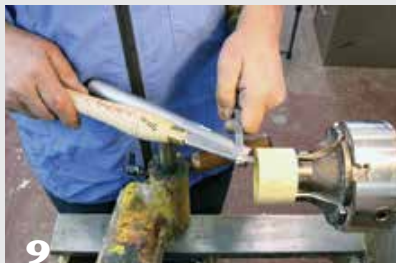
9 The female thread chaser is used with the armrest tool to form interior threads. An initial groove in the chamfer acts as a starting point for cutting the threads. Note that the chaser tool progresses to parallel with the bed ways as the threads develop.
