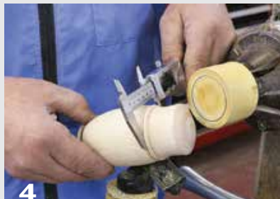
4 A solid prototype is useful for transferring diameters using a caliper. The pencil line on the endgrain shows a target diameter for hollowing the lid.
