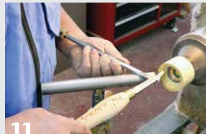
9 The female thread chaser is used with the armrest tool to form interior threads. An initial groove in the chamfer acts as a starting point for cutting the threads. Note that the chaser tool progresses to parallel with the bed ways as the threads develop.
