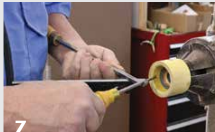
6 The armrest tool (in the author’s left hand) provides cutter access (right hand) inside the lid without having to position the toolrest perpendicular to the lid opening. Form a chamfer at the outer edge, then a recess where the threads will stop.
