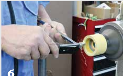
6 The armrest tool (in the author’s left hand) provides cutter access (right hand) inside the lid without having to position the toolrest perpendicular to the lid opening. Form a chamfer at the outer edge, then a recess where the threads will stop.
