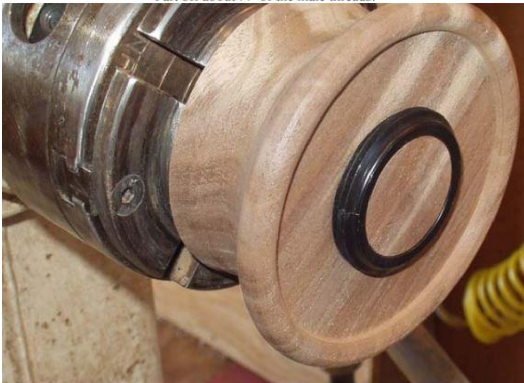
Part off about \frac{1}{4} " of the male threads.
