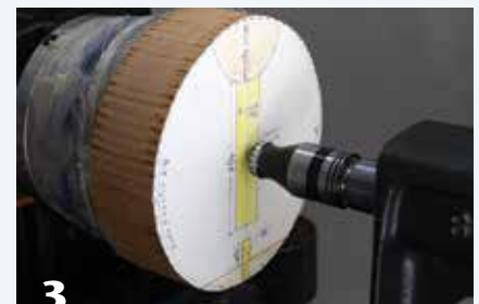
3 After bandsawing the blank round, center it using the point of the tailstock live center for alignment.
