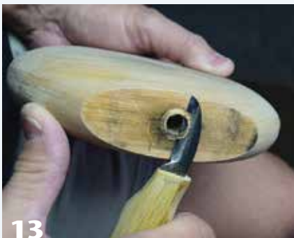
13 Clean up the bottom around the screw chuck hole.
