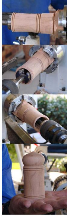
Prepare a jamb chuck the same diameter as the hole drilled in the shaker body, in this case 1 3/8".
