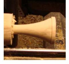
Create a jamb chuck to mount the funnel. I do this to allow me to turn a little depression on the top of the funnel to help salt exit the shaker.
