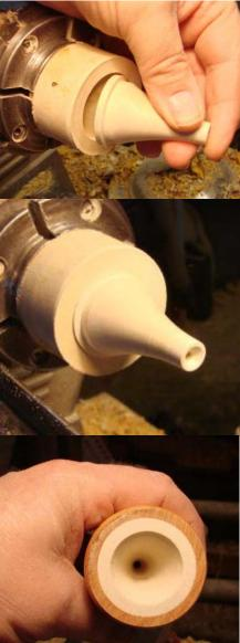
Add a bead of CA glue around the ledge in the body and insert the funnel.
