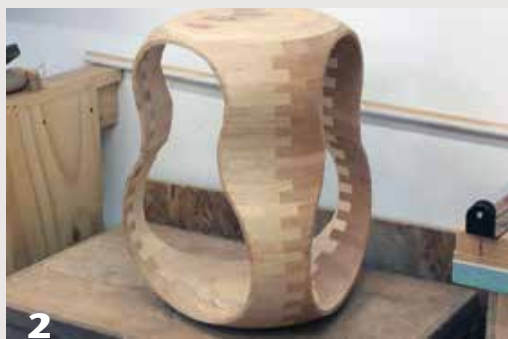
The author's vision: Turn a guitar-shaped vessel, then slice off sections of it to create contoured soundboards.
