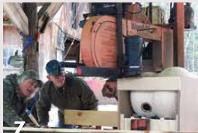
7 The author (right) employs the use of a local sawmill to slab off the three soundboards. Note the specially made jig for holding the vessel safely during cutting.
