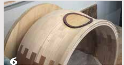
6 A segmented board is turned to thickness, then cut to shape and used as the guitar back.
