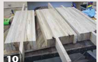
10 The author glues up several boards from which he cuts out the guitar sides.
