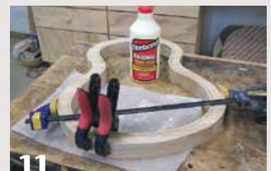
11 To cut out the inside of the form at the bandsaw, a kerf through the side is necessary to provide blade access. After cutting the inside shape, the kerf was closed back up with glue.
