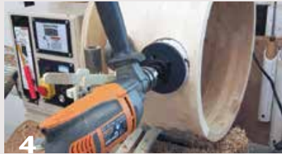
4 The segmented form, once built past the soundhole location, is bored with a hole saw.
