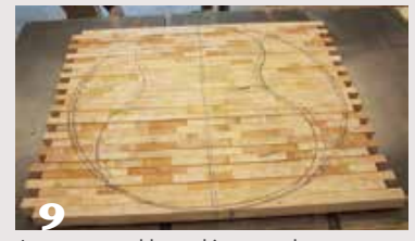
9 To cut out the inside of the form at the bandsaw, a kerf through the side is necessary to provide blade access. After cutting the inside shape, the kerf was closed back up with glue.
