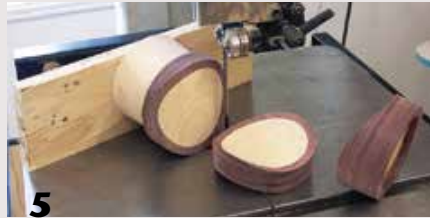
5 Soundhole accents are inserted, then turned flush before construction of the vessel continues.
