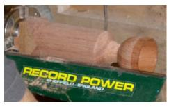
Now the underside of the bowl part can be turned before removing the bulk of the wood to form the basic stem.
