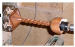
All that remains is to turn on the lathe then part the base from the chucking point and you have made a barley twist goblet.
