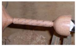
Divide the stem into equal sections using a pencil. The lathe can be turned by hand if preferred but use a soft pencil to make the lines easier to see.
