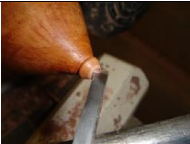
Very carefully, you need to put a dimple in the centre; this will help locate the drill when you end drill.
