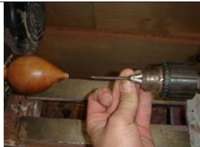
Now I use the closed drill chuck to press a masonry nail into the hole.
