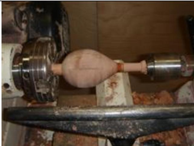
Begin Shaping the bottom of the curve and the tip.
