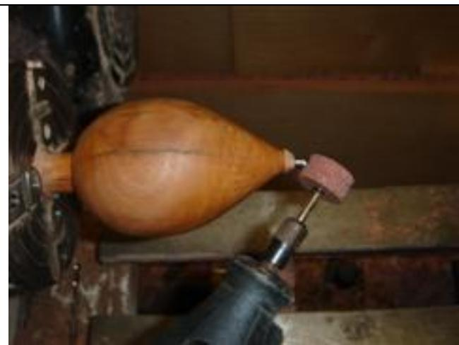
Now take a rotary tool and a grinding wheel, and round off the end of the nail.
