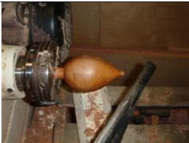
Remove the tailstock and set the tool rest to work on the end.
