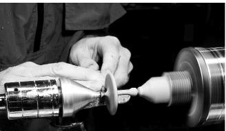
Rosand shapes a small bulbous end on the top of the stem, above left, then refines the shape of the point.
