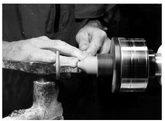
The final shape of the point on which the top spins is done after the tail stock is removed, above left. Then a skew is used to refine the top and part the piece from the lathe.
