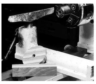
Top Kit: Making tops doesn't require much: a lathe, a wooden disc (you'll find likely candidates in your scrap pile), and a rectangular block. the rest is up to you. Have fun as you shape the disk, the handle and the point on which the unit spins.
