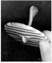
epoxy these pieces together using gap filling epoxy just in case the fit is not perfect. So far I've had no failures.
