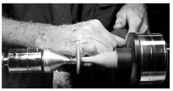
After turning the rectangular blank to a cone shape, above left, the author epoxies it into a hole bored in the disk and begins to refine the shape of the top. The stem protrudes only a half-inch below the disk. Photos by the author.
