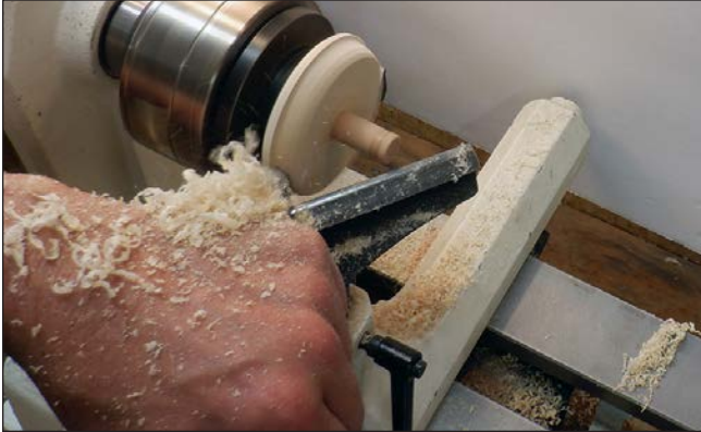
5. Remount — Reverse the workpiece in the chuck to turn the bottom side and spinner point.
