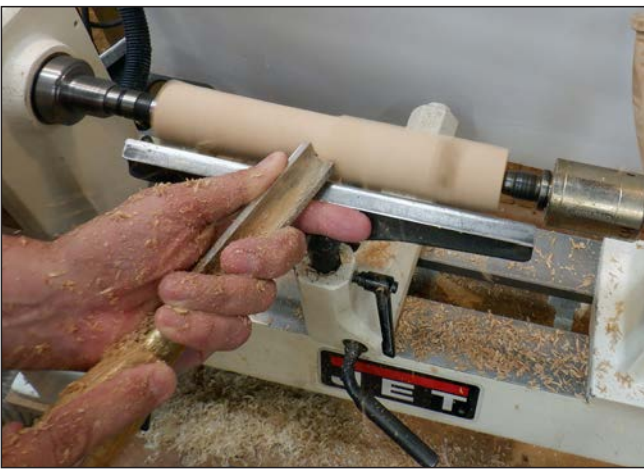
7. Handle — Use the spindle roughing gouge to round the handle blank.
