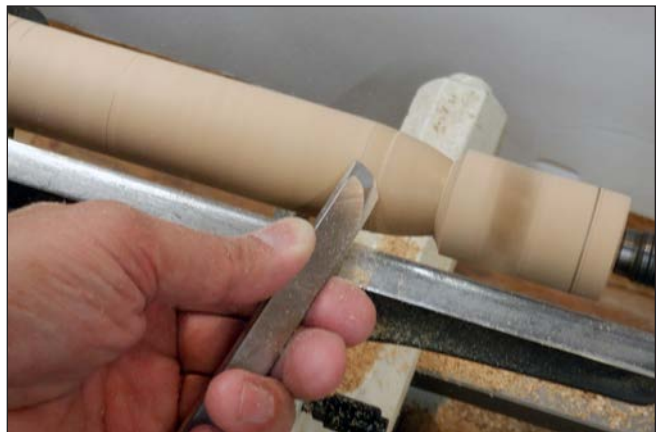
9. Turning the handle — Skew chisel pares the curved shapes.
