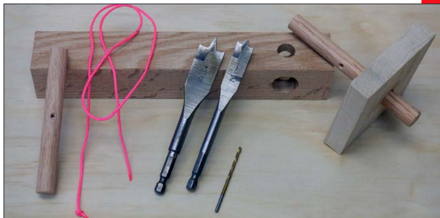
2. Prepared blanks — Bore the spindle blank and dowels as shown, using 3/4" (20mm), 1-1/2" (12mm) and 1/8" (3mm) bits. The wood is red oak (spindle and dowel) and poplar (body of top).
