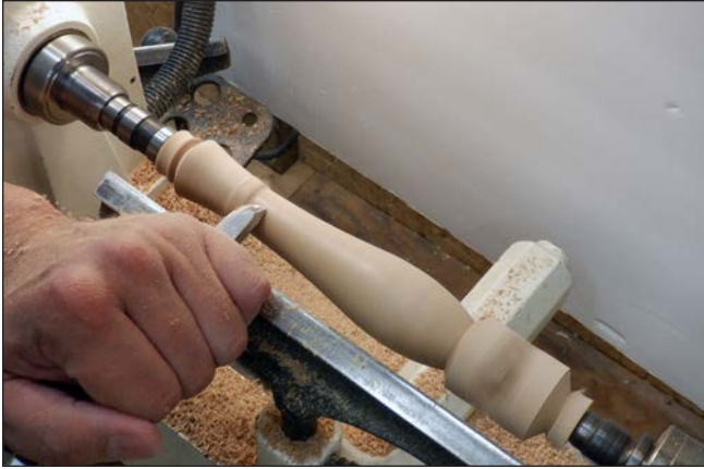
10. Turning the handle — The skew chisel easily cuts a long sweeping curve.
