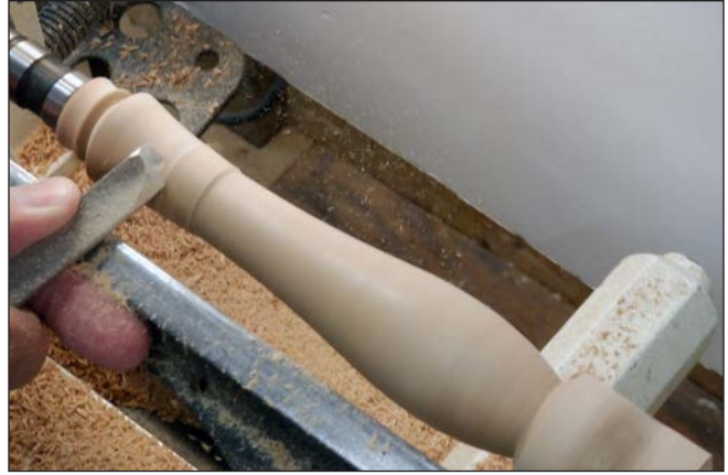
11. Finishing cut — The red oak handle takes a nice texture straight from the skew chisel.
