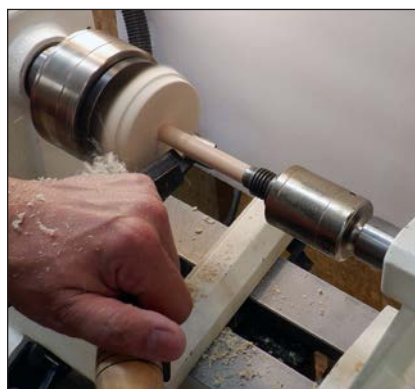
3. Turning the top — With the bowl gouge, cut into the face and toward the headstock.
