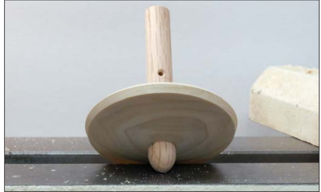
6. Completed top — Sand and finish the wood as you go.
