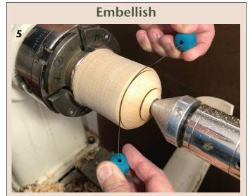
Add burn lines with a wire. A shopmade burning tool is easily made with a short section of wire (a guitar string works well) with beads for handles. Never wrap the wire around your fingers or hands.
