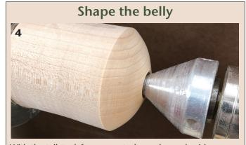
With the tailstock for support, shape the underside.
