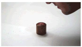
Atmospheric pressure is present around every object on earth. The Newton's Gravity Puzzle is solvable through creating a difference in pressure above and below the inner piece. To overcome the acceleration of gravity, a gentle blow directly on the puzzle will decrease the pressure above the cylinder sucking it out and solving the puzzle.
