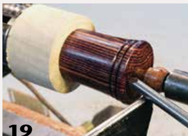
A jam chuck setup for reverse-mounting the base. Note the custom wooden live center, which won't damage the workpiece. A short tenon is formed in the wasteblock to accept the recess in the top of the base. The author uses a point tool to add decorative lines on the bottom.
