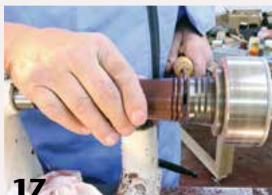
16 Seeing how the spin-top looks when inserted into the base can give you an idea of what the overall design should be. In this case, the author has added two beads at the bottom of the base.
