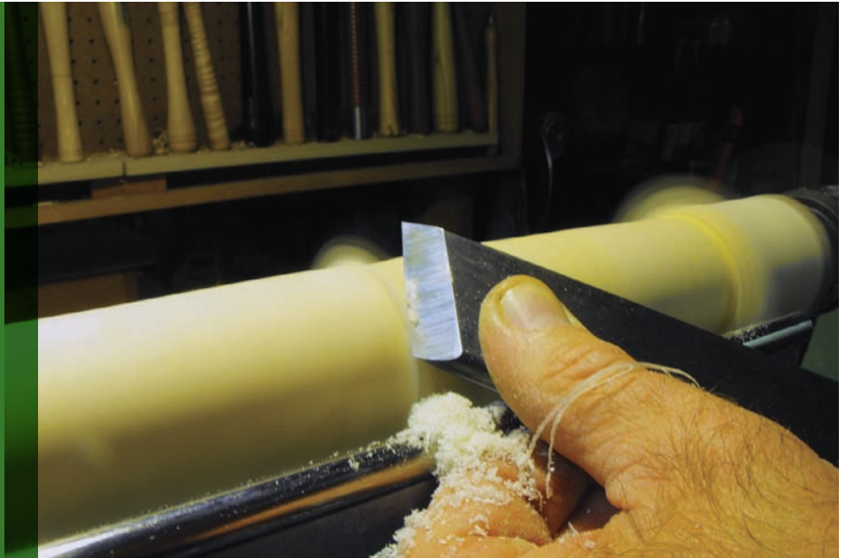
The planing cut, made with the skew chisel's bevel rubbing, leaves a surface requiring minimal sanding.
