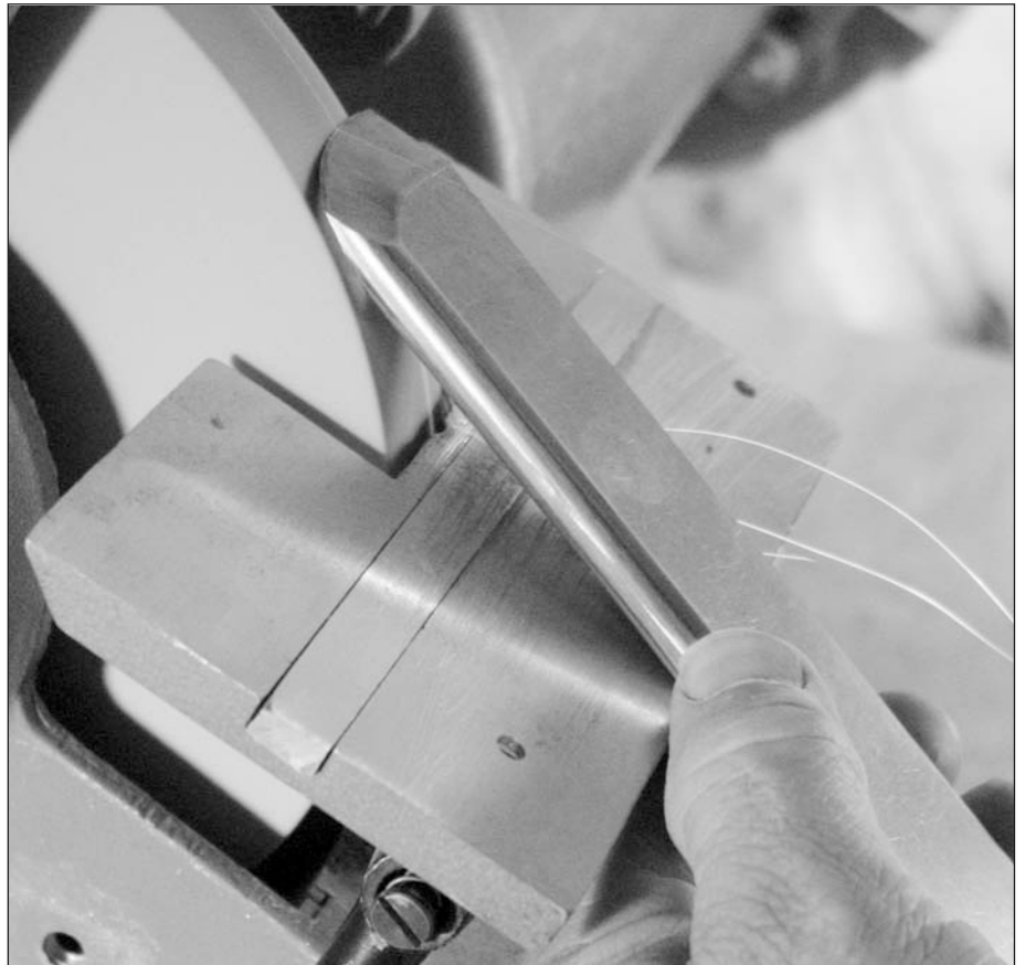
Typical grinding of a skew chisel
