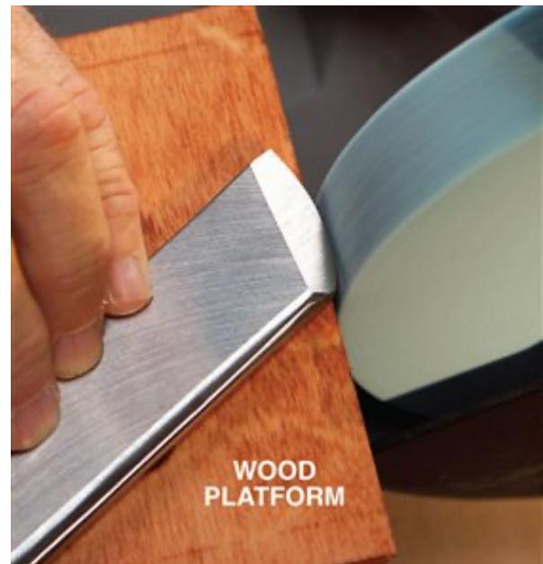
Grind the tool's profile on a 36- or 46-grit wheel (see "The Modified Profile," and Photo 2, right). I use a coarse wheel because this step removes a lot of material.
