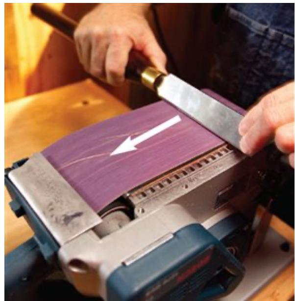
Begin modifying a conventional skew by reshaping its sides (Photo 1). I prefer to do this on a belt sander mounted in a stand and equipped with a belt designed to cut metal (see Sources, below). Be sure to remove all the dust from the sander and set aside its bag to avoid starting a fire. Start with a 60-grit belt; finish with a 120-grit belt. I round the short point side to glide with a smooth motion when planing and to easily rotate and pivot the tool when rolling beads.
