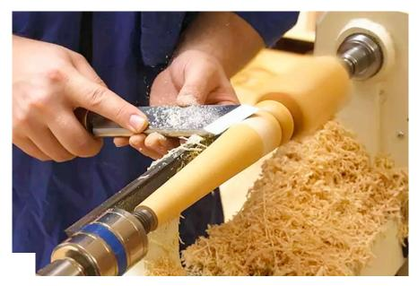
Interested in spindle turning? Then come along and discover the keys to effectively sharpening and using the indispensable skew chisel. You'll soon be producing fine, ribbonlike shavings and superbly smooth surfaces in need of little sanding.
