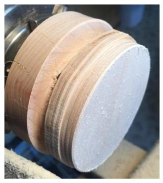
Here's a picture of the rotary disk being rounded while mounted on the screw chuck. Note the lack of a hole in the front side. Once I got half the disk rounded true, I dismounted the disk from the screw chuck and mounted it in grooved jaws to cut the back-side bevel.
