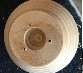
At this point, your bearing assembly is installed in the sanding disk, and this step is finished.
