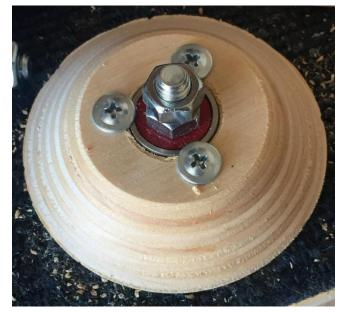
Once the bearing spins freely, remove it, and drill three pilot holes for the retainer screws that will hold the bearing and bolt head in place. You want the head of the retainer screws to reach out over the outer bearing race, but not much further, lest you compress the sealed bearing cover.
