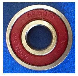
Here is the "top" side of the bearing. You can see the red rubber seal that will keep sawdust out of the bearing race. The backside does not have the rubber seal, but it is "buried" in the rotary sanding disk where no sawdust should reach it.
