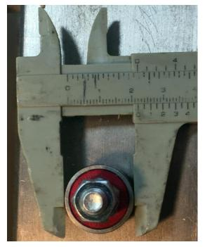
You can set your calipers to 22 mm, or you can run the jaws up against the bearing, and the calipers will set themselves at 22 mm. Even cheap plastic calipers can do this. Look carefully, and you'll see they are exactly on 22 mm.
