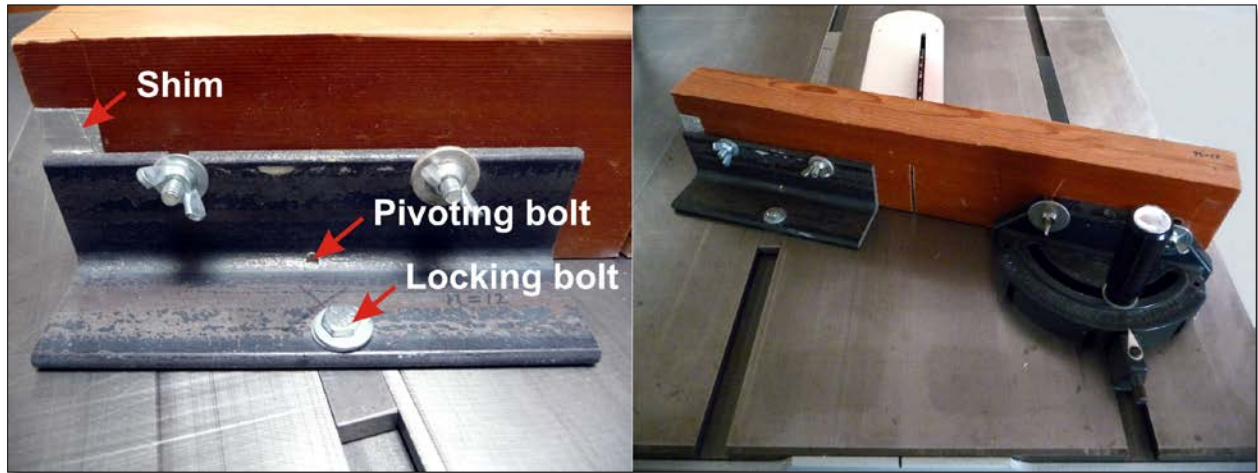
Figure 3. Miter gauges for cutting segments on a table saw.
