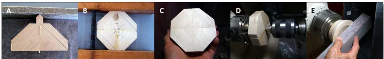
Figure 4. Making the foot (first layer). A: Gluing two quadrants together; B: Gluing two halves together after the facing surfaces are trued up; C: One side sanded flat on a disc sander; D: Tailstock used for centering/holding onto the waste block after glue is applied; E: Truing up the first layer. Note the center has been dished out for easy truing.
