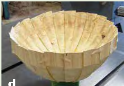
d Glue the twenty-four staves together, and turn the bowl.
