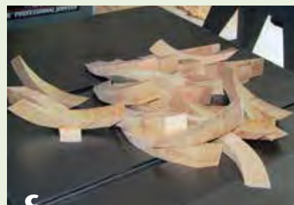
c Cut the staves at the bandsaw, with the table tilted to 7.5 degrees.
