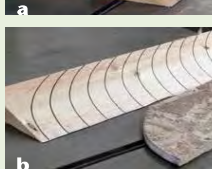
a b Mark the staves on the wedge-shaped board using a pattern, so all the staves are the same shape and size.
