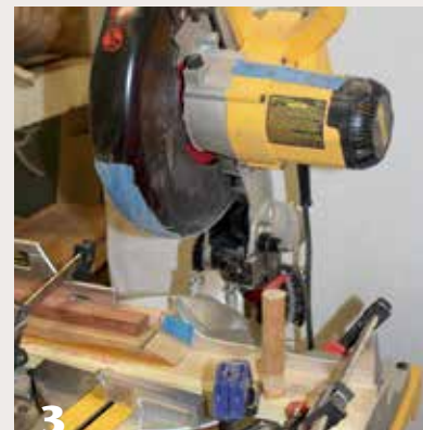
The author's jig for cutting segments on a compound miter saw. A slope adjacent to the cutline allows the segments to fall away safely.
