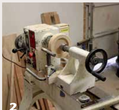
The vase is assembled on an MDF base, which is mounted in a chuck.
