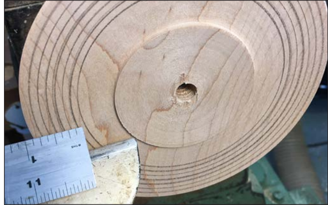
Photo 2. Using a pencil and ruler, mark off even divisions for the beads.
