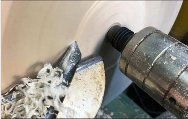
Photo 1. After chucking the form by its foot, face off the top and smooth the outside with shearing cuts.
