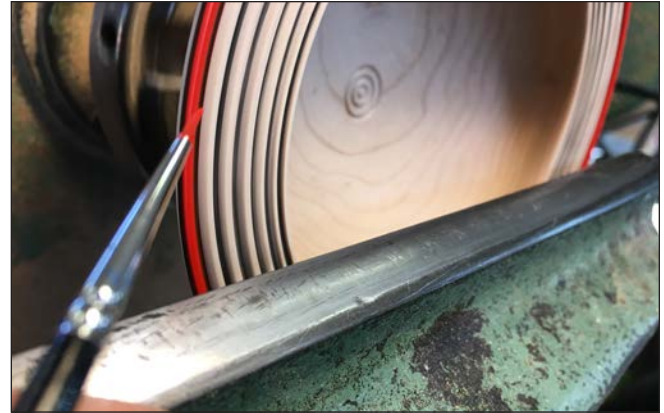
Photo 13. Rotate the lathe slowly to apply an even coat of paint. Reversing the rotation ensures even coverage.
