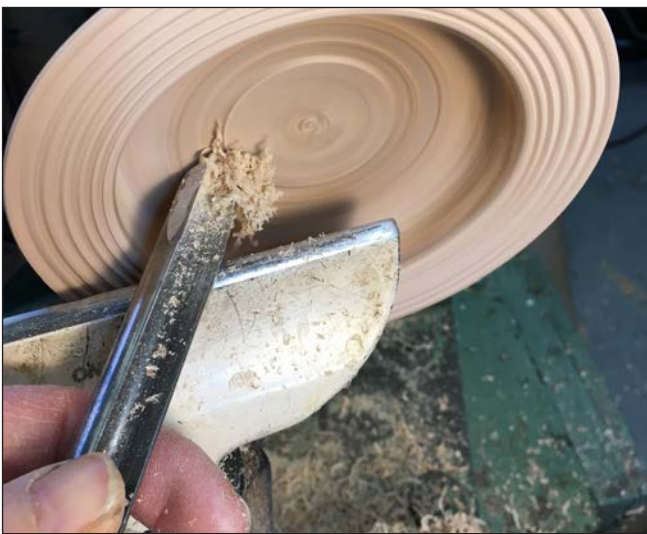
Photo 7. Complete the hollowing using a bowl gouge and scraper.
