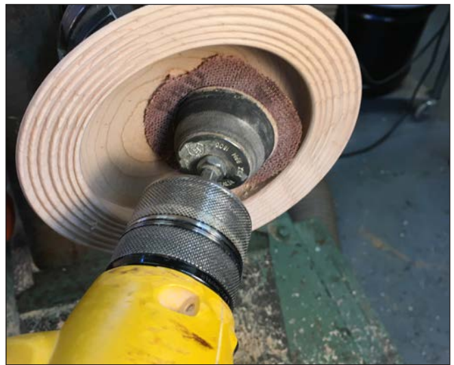
Photo 8. Sand the interior. The over-sized disk conforms with the curve of the undercut rim.
