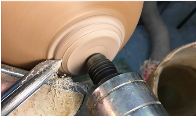
Photo 17. Shape the foot with a detail gouge, and add any decorative embellishments.
