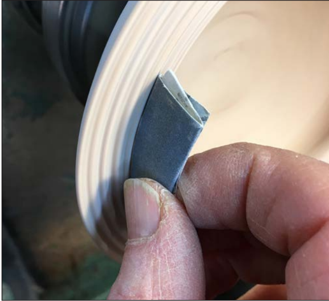
Photo 9. Sand the beads by hand to preserve their shape. Beads sand quickly, so don't be too aggressive, especially with coarse grits.
