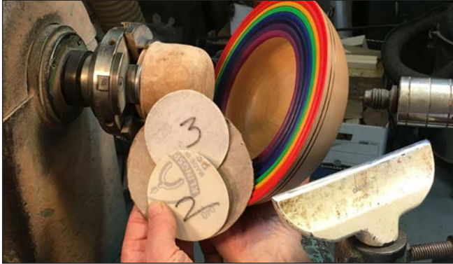
Photo 16. Use a vacuum chuck or a jam chuck with abrasive disks to access the foot for final turning.
