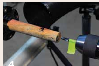
4 Ready to drill the hole for the stem. A tape flag added to the drill bit indicates proper depth.
