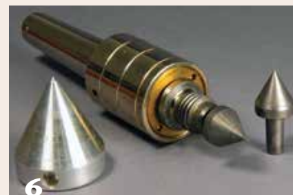
6 A typical tailstock live center and the oversized stock cone at left. For smaller projects, the author prefers a penturner's point shown on the live center and at right.
