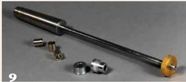
This kit requires a penturning mandrel, with bushings and spacers.
