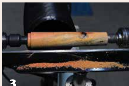
3 Handle roughed between centers, with a tenon formed so it can be held in a chuck for drilling.
