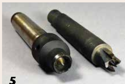
5 Two styles of drive centers, left is a cup center and right a small prong center. Choose a drive sized for your work.
