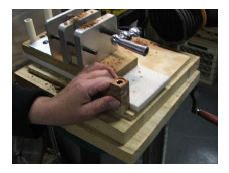
.What the blank will look like after trimming with the barrel trimmer.
