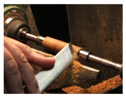
Turn the blank down to the bushing. **REMEMBER**, you can always sand a little more off, but you can't put it back on! Shape the pen barrel to your liking.
