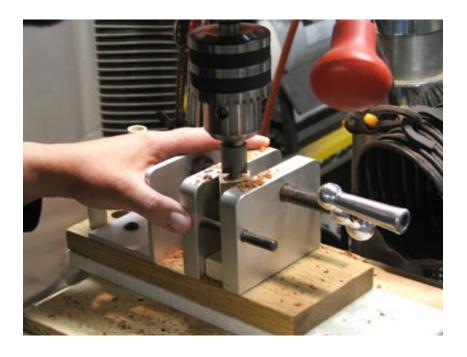
After the glue dries, trim the pen blank (if instructions require it) until the brass shows. Using a barrel trimmer and vise will insure the best results.
