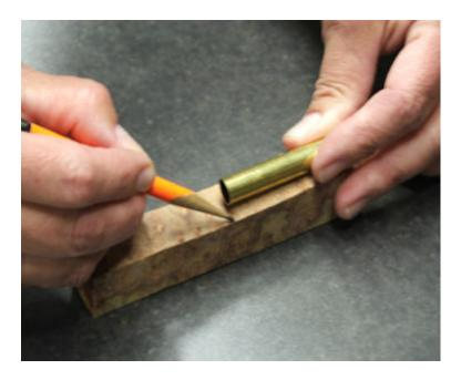
Following your instructions, mark your pen blank for cutting to the correct size. Most kits require the wood blank to be 1/8" or so longer than the brass tube for squaring up later. Read the instruction sheet to make sure.
