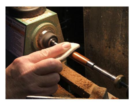
Use a buffing pad between coats. If wax ridges appear, try buffing pad to remove. If not successful, you may have to use the white 3-m pad which will require you to reapply the polish and wax again.
