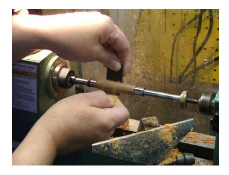
.Sand the pen barrel going through the grits. In between grits wipe away any excess sawdust and check for sand paper "rings". If they appear, sand horizontally (with the lathe off) before proceeding onto the next grit.
