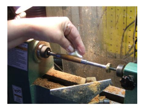
If you are happy with your sanding, apply 2 coats of friction sanding sealer with a small lint free rag. This will raise the grain and remove any fine sawdust in the pores of the wood.
