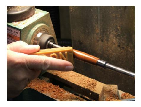
.Apply 3-4 coats of carnuba wax. Constant horizontal movement of bar will help prevent wax ridge buildup.
