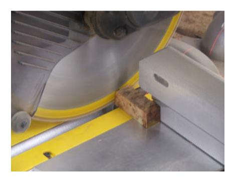
Cut the pen blank to size with a band saw, scroll saw, chop saw, table saw, or a hand saw for that matter....use what you are comfortable with.
