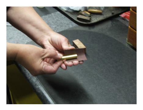
Using a coarse grit sand paper (80 will do) to sand the brass tube. The Small grooves the sanding leaves will give the glue something to bond to.
