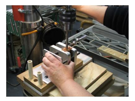
Find the center of your pen blank and drill it out with the appropriate bit called for in your instruction sheet. Use a vise to insure you drill the hole straight. Make sure you only drill 1/2" at a time before clearing chips from the hole. Continue this until you drill completely through the blank.
