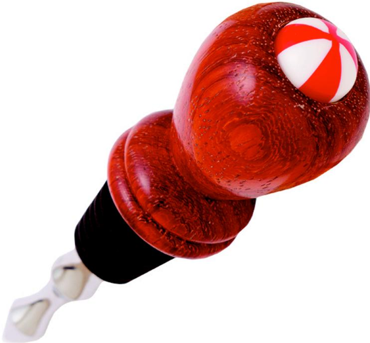
Use a small piece of contrasting scrap wood, plastic or Corian™ to make a unique Cabochon insert that adds interest and design your [bottle stopper](#) project. First determine the diameter of the cabochon. It can be as small as 1/2" or as large as 1-1/2" (3/4" cabochon shown in the photos).
