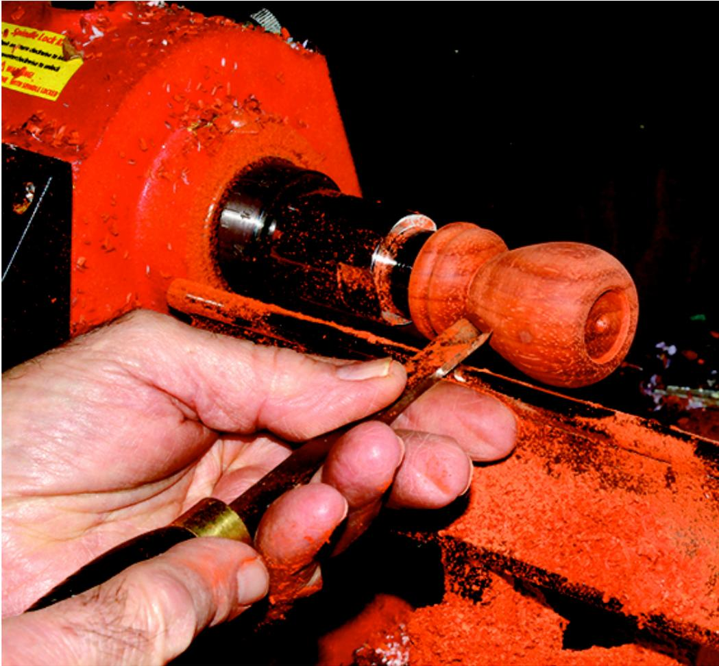
Penn State Industries carries a dedicated [pen blank drilling chuck](#) that is ideal for turning a pen blank into a cabochon up to 1" in diameter. Place a pen blank (can be a short piece of pen blank scrap) in the chuck. Turn a dome to about 1/4" high at the end of your blank, match the diameter to the recess you drilled in the [bottle stopper blank](#). Finish and polish the cabochon dome, part it off of the blank, then glue it into the recess in the stopper blank.
