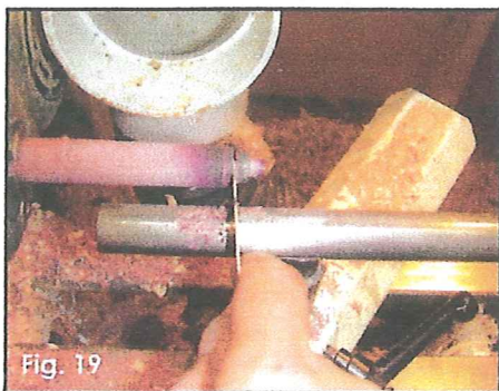
Fig. 19 Singe the wood after cutting the tenon to final size.
