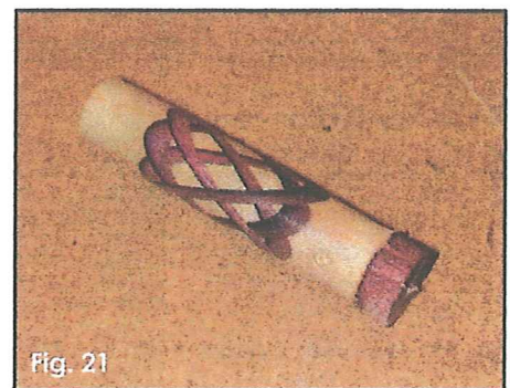
Fig. 21 Glue in the rough finial in preparation for final turning.
