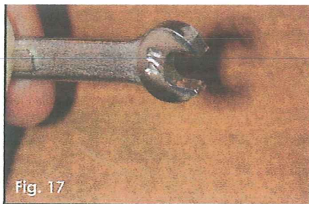
Fig. 17 Tenon tool made from a wrench.
