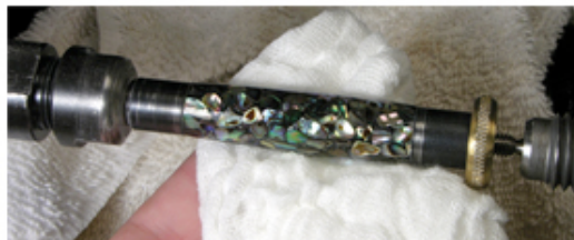
Photo 14 Use a soft cloth to polish the blank
