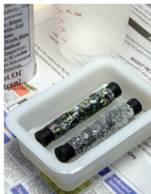
Photo 6 Place the plugged tubes into the hardened mold
