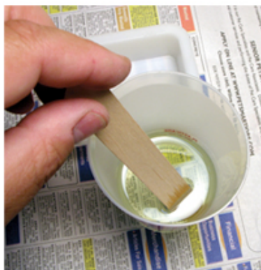
Photo 3 Mixing the Resin
