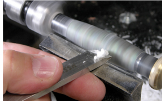
Photo 12 Turn blank down to bushings
