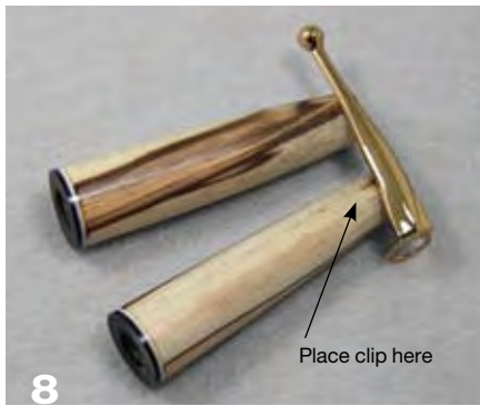
8 By planning ahead, you can place the pen clip over ordinary wood grain.
