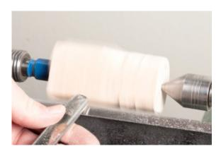
Turn the blank to round with a roughing gouge. Now we need to cut a tenon on one end of the blank to mount in a
