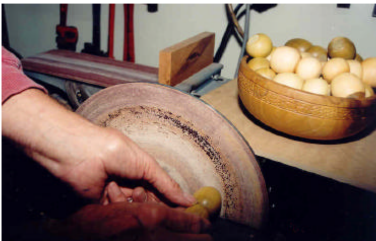
Self explanatory - 100 grit on my Disc/Belt sander combo
