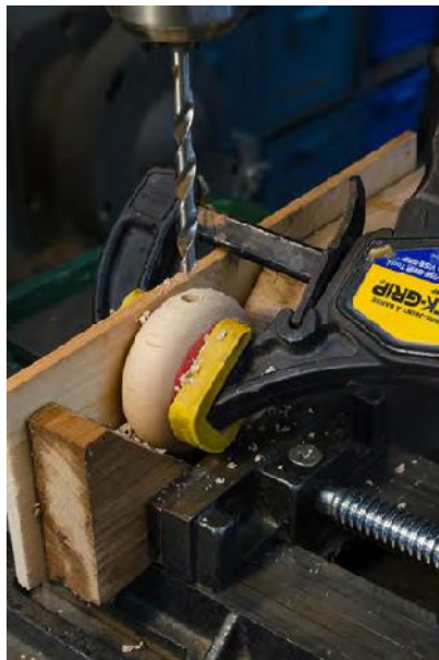
Photo 12 - To safely drill the hole through the ornament, build a V jig.
