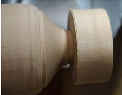
Photo 2 - Reduce the diameter 1" from the end to a little less than 1".
