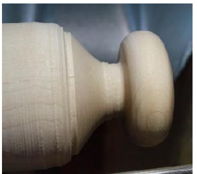
Photo 4 - Shape the ornament using a spindle gouge.
