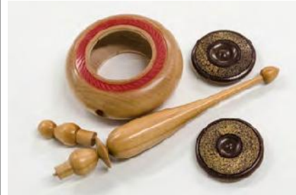
Photo 19 - The parts are turned and ready to be assembled.
