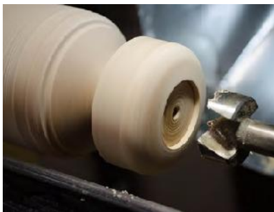
Photo 3 - Use a Forstner bit to create a 1/8" deep recess.
