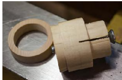
Photo 8 - Prepare the expansion, or collet, chuck blank by turning a tenon on each end. (The ring moves the ornament out a little so the collet chuck works better.)
