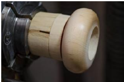
Photo 10 - By tightening the screw, the collet jaws expand and hold the ornament securely.
