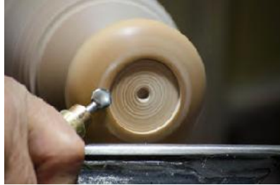
Photo 5 - A texturing tool can be used to create a pleasing design on the side of the ornament.
