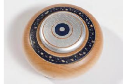
Photo 21 - A simple ball cutter attached to a drill can create interesting designs.
