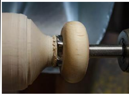
Photo 7 - Use the Forstner bit to drill all the way through the ornament.
