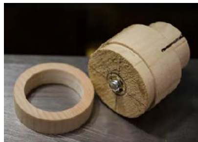
Photo 9 - Drill a 5/16" hole through the collet chuck to accommodate a threaded insert.
