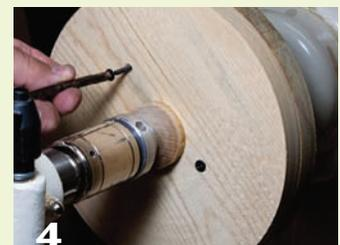
4 Screw the two disks together and carefully true up the assembly.
