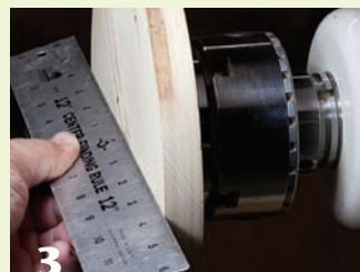
3 Make sure the face of each disk is flat, so they can later be glued together securely.
