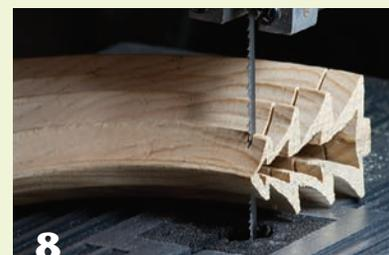
8 With the outside profiles turned and the center of the disk parted off, saw out the trees.
