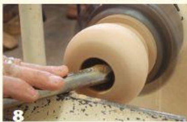
8 After the outer shape is finalized, hollow out the globe or shell.
