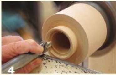
4 Cut the recess for the legs.
