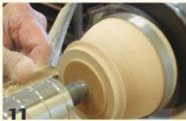
11 Reverse the shell in the chuck, expanding a set of chuck jaws inside the hole made for the base. (There was a small crack in the wood, so I used a hose clamp to prevent the shell from splitting.)
