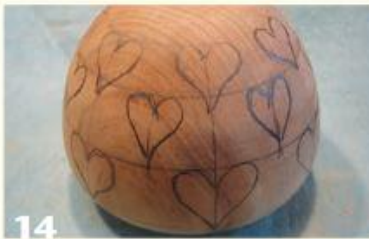
14 Lay out the pattern of the openings you wish to pierce through the shell.
