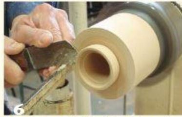
6 When you are satisfied with the size and shape of the base and have achieved a tight fit for the light, sand the base smooth and part it off using a thin parting tool.
