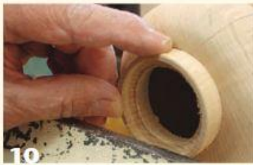
10 Check the fit of the base to avoid oversizing the opening. A slight taper in the opening will help achieve a tight fit. The joint is simply wood-to-wood, no shoulder. Sand the bottom area of the shell and base.
