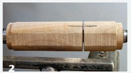
Rough-turn the blank and turn tenons on both ends. Make a partial parting cut where the lid and bottom will be separated and finish the cut off the lathe. Make a reference mark for future alignment.
