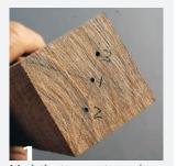
Mark the true center and label it 1. Then add two other axis points ½" away, labeled 2 and 3. Do this on both ends of the blank.
