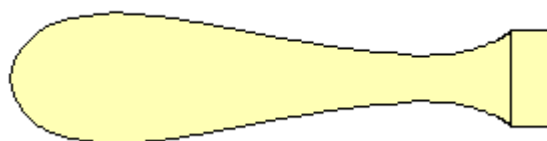
Diagram 8.4 Blending a bead and a cove to form a handle shape
