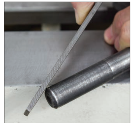
Chamfer. Relieve the end of the toolrest post so it easily enters the post hole.
