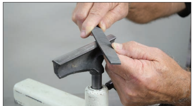
Toolrest. Draw a file with both hands over the full length of the toolrest to remove any dings.
