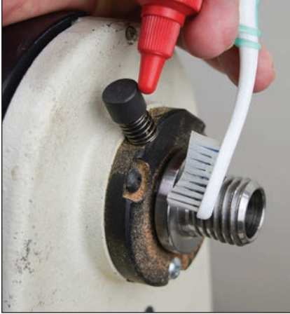
Locking pin. Clean and dry-lube the locking pin and spring.
