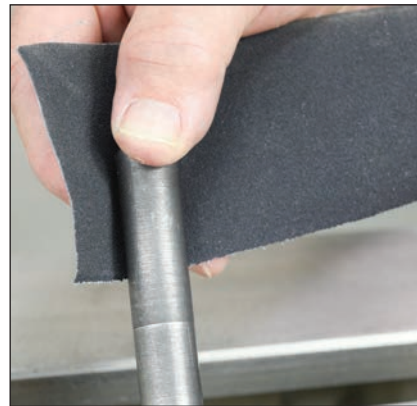
Toolrest post. Remove dings on the toolrest post with emery cloth, or a file.
