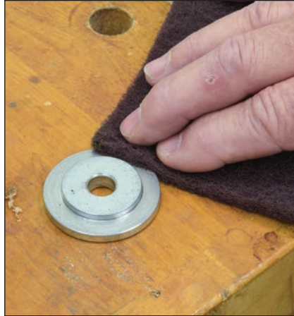
Locking plate. Locking plates can be circular or rectangular. They should be cleaned, but not waxed or lubricated.
