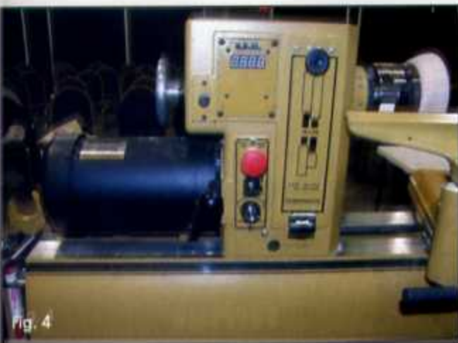
Fig. 4 Here is a close-up of the headstock and lathe controls. Note how the headstock is able to be moved along the bed of the lathe. By positioning it along the bed as needed, you can make a short-bed lathe, spindle lathe, and anything in between!
