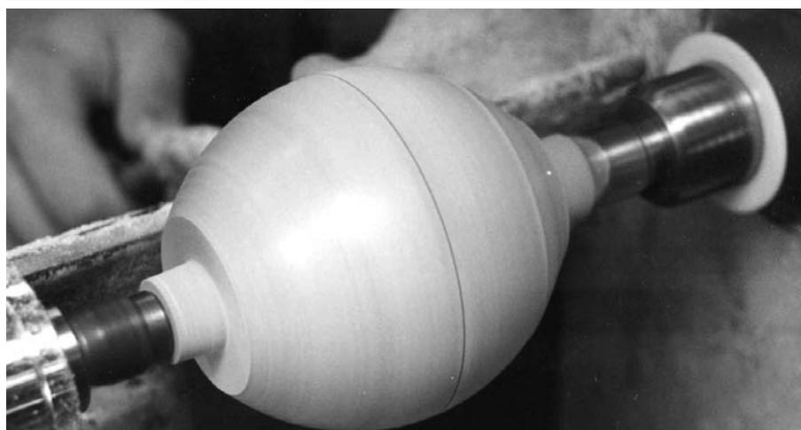
After turning the blank to a cylinder and marking its centerline, the author gauges roundness with a plastic ring (top photo). The visible gap shows the sphere is slightly elongated, requiring removal of more material (bottom photo). Photos by Hal Simmons
