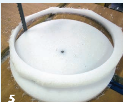
5 Use the jig to cut a circle from the cutting board.
