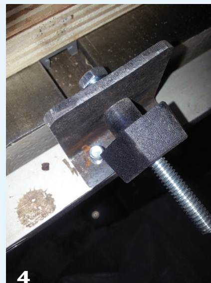
4 A bolt threaded through a piece of angle iron makes a stop to fine-tune the jig's alignment.
