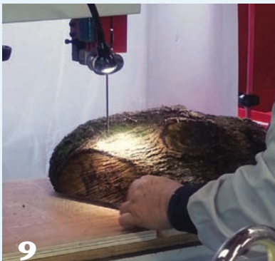
9 The jig allows you to rotate the blank smoothly into the blade.
