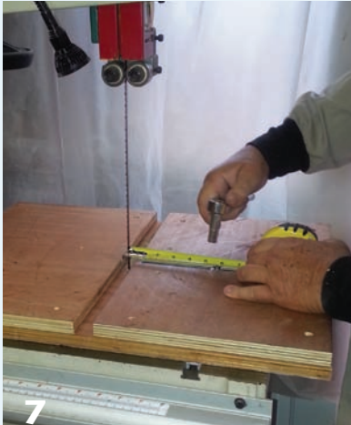
7 Measure the radius of the blank to be cut and use a socket wrench to lock the pivot pin at that point.
