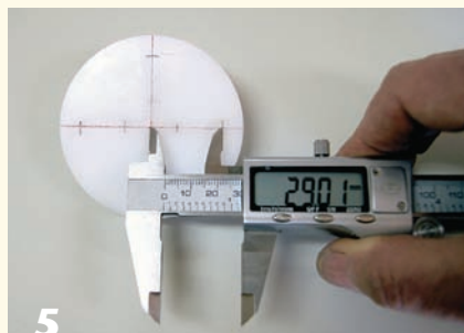
Precisely mark the location of the mounting screw holes. First drill the shank holes, then countersink to recess the screw heads.
