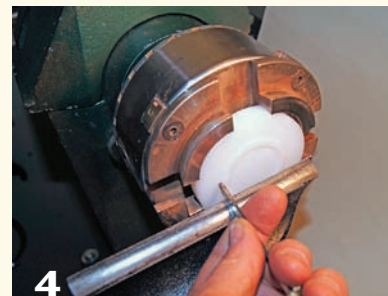
A parting tool is used to form the circular tenon, used later for mounting the jaws to the chuck.
