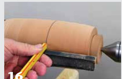
16 Mark the curve change point on the vase, then turn it to your desired shape.
