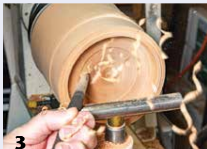
3 This hollowing is into endgrain, so the author cuts from center outward to the left. Avoid vibration by hollowing and shaping the outside wall incrementally, rather than hollowing all at once.
