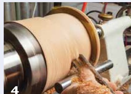
4 A padded platter mounted to a faceplate on the tailstock provides great support at the open end of the hollowed base section. A simple piece of plywood with a craft foam pad would work well, too.
