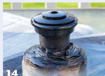
14 The lid is turned, threaded, and painted. Notice the \frac{3}{8} " (10mm) hole to accept the finial later. Part of the length of threads will be cut away to provide a reasonable thread engagement.
