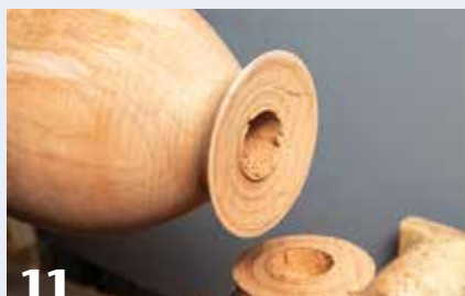
11 With the urn remounted on the lathe, the top end is parted off within the pre-hollowed depth.
