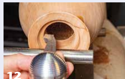
12 After cleaning up the top of the urn and filling any exposed cracks, the inner diameter of the neck is formed, a recess cut, and threads chased.
