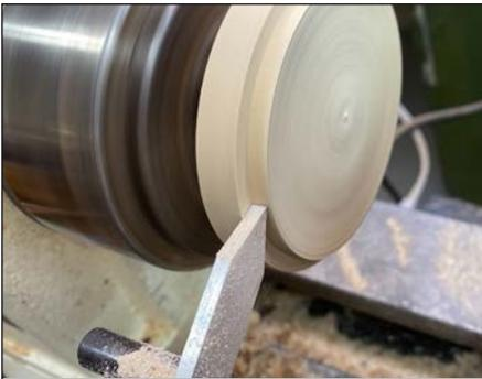
Use a parting tool to cut a tenon *almost* down to the line.
