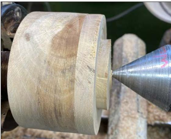
When the top fits, re-chuck the box and use it as a jam chuck to finish the top. If the top is too loose to stay on the
