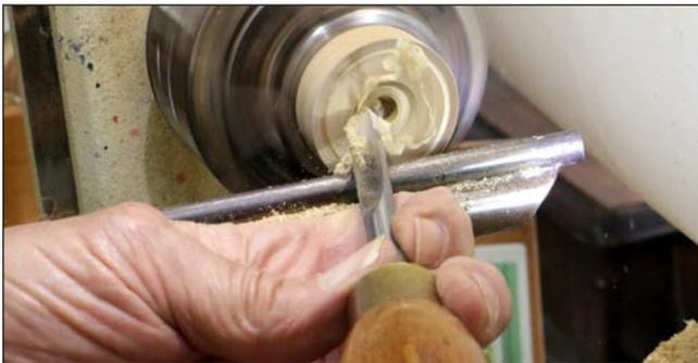
Remove the wood from the center of the lid working from the hole in the center to just shy of the caliper line. Here I use a 3/8" spindle gouge.
