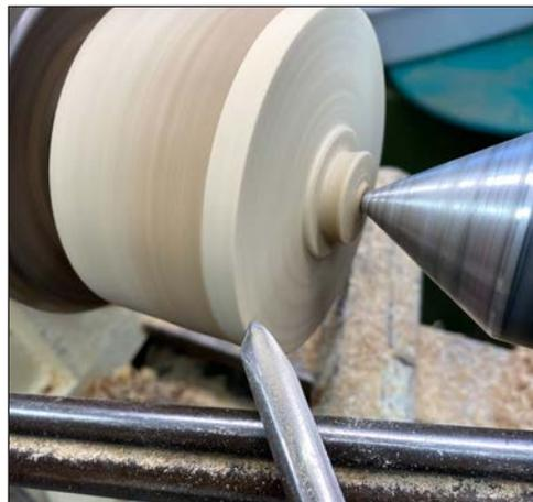
box, a piece of paper towel in the joint should snug the fit. Bring up the tailstock while turning the top of the lid.
