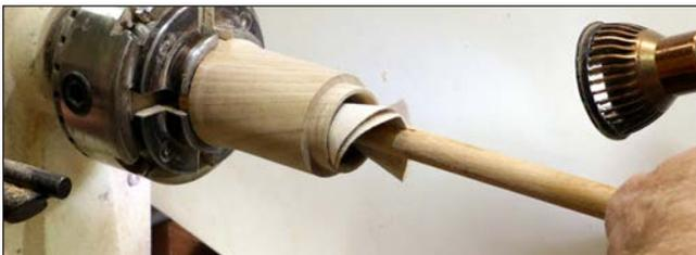
Sand and finish the inside of the box. Lightly sand the tenon. For safety, the narrow interior of a box should be sanded by wrapping a piece of abrasive around a dowel, rather than sticking your fingers in the spinning blank.
