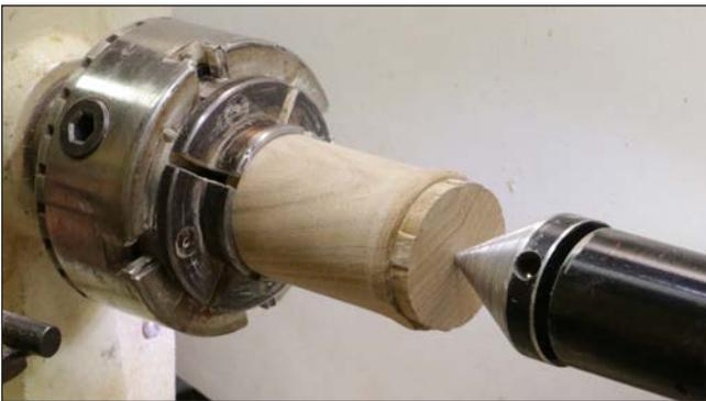
Re-chuck the box and use it as a jam chuck to hold the lid. Finish turning the top of the lid. To finish the bottom of the box, reverse its orientation on the lathe and gently clamp the tenon on the top of the box in the scroll chuck. If you are concerned about marring the tenon, wrap a layer of shop towel around it before snugging the chuck jaws. Bring up the tailstock and engage the live center. Take light cuts to remove the bottom tenon, and finish the bottom.
