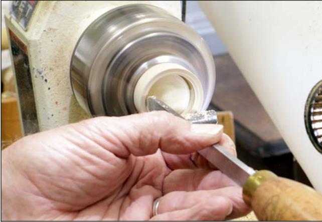
Finish hollowing the lid to the depth of the drilled hole. Use a parting tool to square the mortise to the final depth. Sand the inside of the lid but don't sand the sides of the mortise unless the fit to the box is too tight. Just a little sanding with 240- or 320-grit sandpaper can change the fit of the lid to the box.
