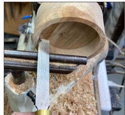
Cut the box's walls parallel with a flat-end scraper so that the lid will fit properly.
