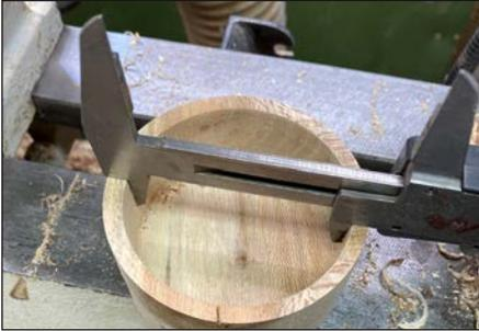
After hollowing, sanding, and finishing the box's interior, use a Vernier caliper to measure the interior diameter.
