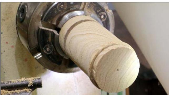
Cut a slight taper in the lid from the mark left by the caliper to the bottom of the 1/8" hole.
