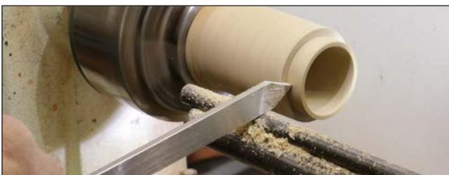
Hollow the box and use a parting tool to create the tenon at the top. Make the tenon about 3/8" (10mm) long.
