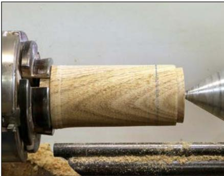
Rough the blank between centers and put a tenon on both ends. In this case, the grain is running parallel to the lathe bed.
